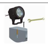
Fixing the Led luminaire with screws of maximum diameter 8mm
