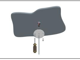
Fix the rosette by screws with maximum diameter 4mm
