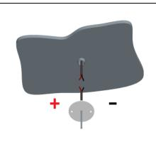
Carry out the electrical connection respecting the polarity of the cables
