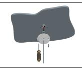
Fix the rosette by screws with maximum diameter 4mm.
