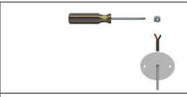
Define the length of the suspension and fix the cable stopper on the cable of the suspension by screwing the screw.
