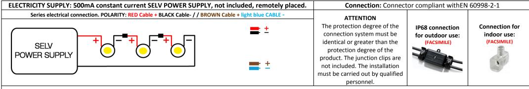
• ATTENTION: Before starting all electrical connections, make sure that the power supply is not powered. The connection to the electricity grid must be carried out only after completing the wiring of all the components. If this simply rule is not respected, the lighting source will be irremediably damaged. The installation must be carried out by qualified personnel.
