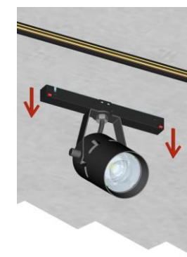
Traction release of the "Duomo Mini" product from the track
