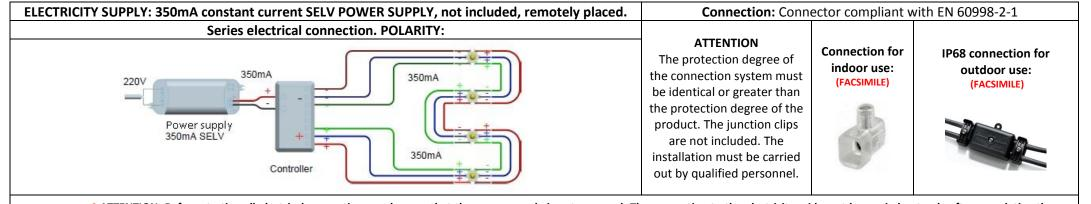
• ATTENTION: Before starting all electrical connections, make sure that the power supply is not powered. The connection to the electricity grid must be carried out only after completing the wiring of all the components. If this simply rule is not respected, the lighting source will be irremediably damaged. The installation must be carried out by qualified personnel.
