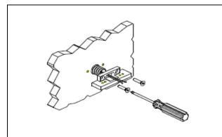
Fix the support to the wall with countersunk screws (diameter 4 mm). Screws not supplied by us.
