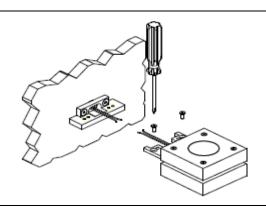
Carry out the electrical connection paying attention to the polarity of the cables
