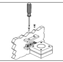
Fix the lamp to the support with the screws provided
