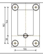
Fix the magnets to the wall with countersunk screws 4mm diameter (screws not supplied by us).
