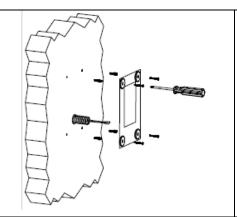
Mark the fixing points of the magnets through the template supplied by us
