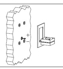
Carry out the electrical connection paying attention to the polarity of the cables.
