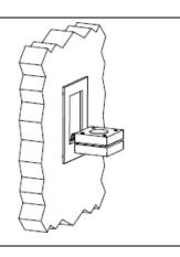
Lean the lamp on the magnets, making sure that they insert into the specific housings.
