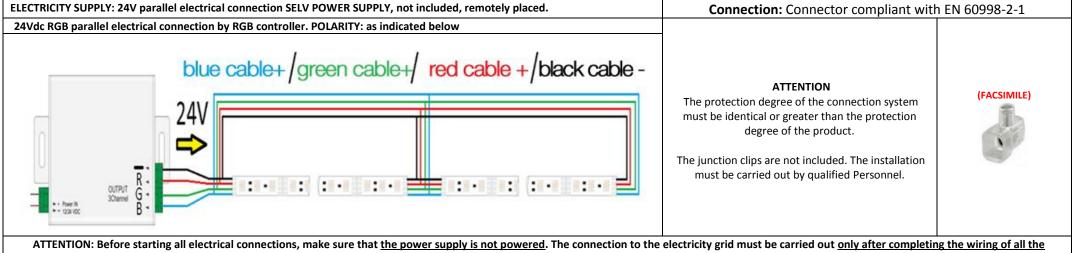
ATTENTION: Before starting all electrical connections, make sure that the power supply is not powered. The connection to the electricity grid must be carried out only after completing the wiring of all the components. If this simply rule is not respected, the lighting source will be irremediably damaged. The installation must be carried out by qualified personnel.
