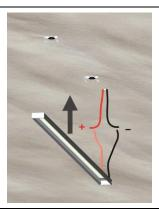
Carry out the electrical connection and insert the bar on the brackets
