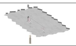
Fix the supports for the hook maintaining a straight line
