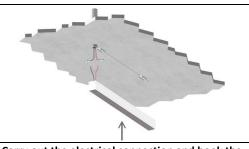
Carry out the electrical connection and hook the bar
