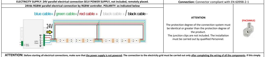
ATTENTION: Before starting all electrical connections, make sure that the power supply is not powered. The connection to the electricity grid must be carried out only after completing the wiring of all the components. If this simply rule is not respected, the lighting source will be irremediably damaged. The installation must be carried out by qualified personnel.
