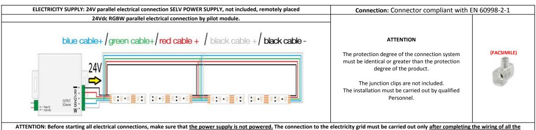
ATTENTION: Before starting all electrical connections, make sure that the power supply is not powered. The connection to the electricity grid must be carried out only after completing the wiring of all the components. If this simply rule is not respected, the lighting source will be irremediably damaged. The installation must be carried out by qualified personnel.
