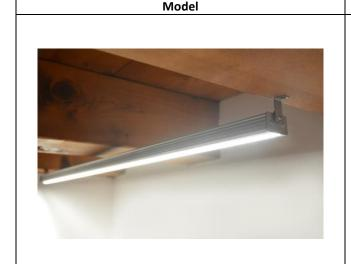
On wall/ceiling Clam Led Bar with single or double light emission. Finish: black/grey anodized aluminum. Screen: opal/semi-opal/transparent. Stainless steel terminals. It is provided with 25cm bipolar cable for the electrical connection. Maximum length 2000mm (longer lengths on request). Indoor installation on any rigid surface by suitable "L" brackets. Fixing with two screws suitable to the support not supplied by us.
