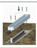
Carry out the electrical connection and fix the bar with screws
