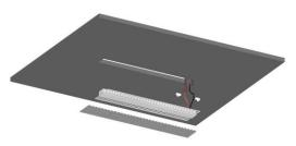
Insert the bar and fix it with suitable small net. Carry out the electrical connection respecting the polarity
