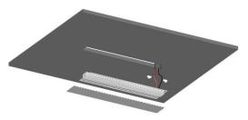
Insert the bar and fix it with suitable small net. Carry out the electrical connection respecting the polarity
