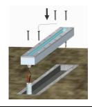
Carry out the electrical connection and fix the bar with screws
