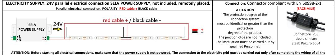
ATTENTION: Before starting all electrical connections, make sure that the power supply is not powered. The connection to the electricity grid must be carried out only after completing the wiring of all the connection to the electricity grid must be carried out only after completing the wiring of all the connection to the electricity grid must be carried out only after completing the wiring of all the connection.
