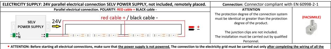
• ATTENTION: Before starting all electrical connections, make sure that the power supply is not powered. The connection to the electricity grid must be carried out only after completing the wiring of all the connection to the electricity grid must be carried out by qualified personnel.
