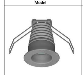
Ceiling recessed Led light body in aluminum, 14mm backward light source. Finish: silver grey anodized aluminum, other colors on request. On request, also other materials for the visible part: stainless steel, brass, etc. Screen: transparent polycarbonate. It is provided with 25cm cable for the electrical connection to the pilot module. Indoor installation on any rigid surface, fixing by torsion springs.
