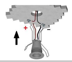
Carry out the electrical connection respecting the cables polarity. Insert the spotlight in position.
