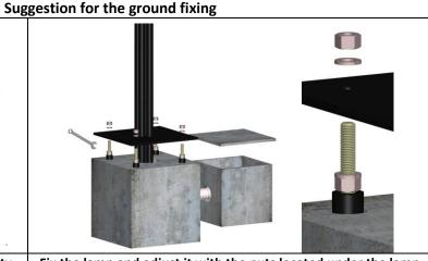
Fix the lamp and adjust it with the nuts located under the lamp plate
