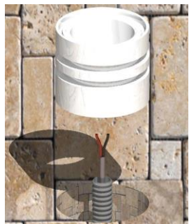
Position and fix the formwork flush with the floor
