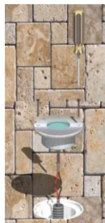
Carry out the electrical connection paying attention to the cables polarity and fix the lighting body with 2 screws
