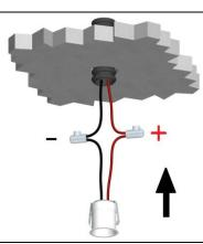
Carry out the electrical connection respecting the cables polarity.
