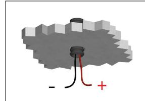
Drill the hole **Ø22**mm with 1mm chamfer on the edge
