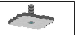
Carry out the housing hole Ø35mm
