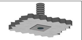
Carry out the recess hole Ø35mm
