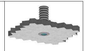
Carry out the housing hole Ø36mm
