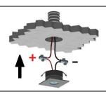
Carry out the electrical connection respecting the cables polarity.
