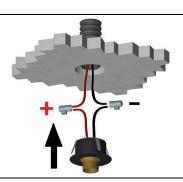
Carry out the electrical connection respecting the cables polarity.
