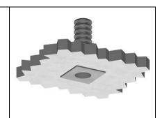
Carry out the housing hole Ø36mm
