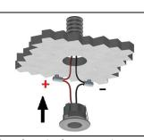
Carry out the electrical connection respecting the cables polarity. Insert in position
