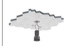
Carry out the electrical connection paying attention the cables polarity and insert in position the spotlight
