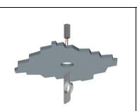
Drill the hole 50mm diameter for housing of the formwork
