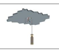
Insert of the formwork and fix it in the drywall with two self-tapping screws
