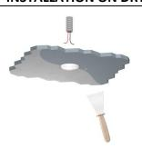
Carry out the finish of the ceiling being careful to keep the spotlight housing perfectly clean
