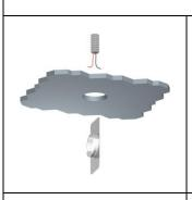
Drill the hole Ø75mm and insert the formwork
