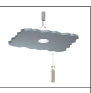
Fix the formwork on the drywall with two self-tapping screws
