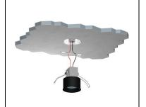
Carry out the electrical connection respecting the cables polarity.
