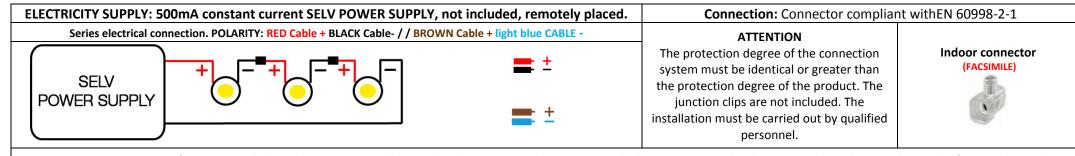
• ATTENTION: Before starting all electrical connections, make sure that the power supply is not powered. The connection to the electricity grid must be carried out only after completing the wiring of all the components. If this simply rule is not respected, the lighting source will be irremediably damaged. The installation must be carried out by qualified personnel.
