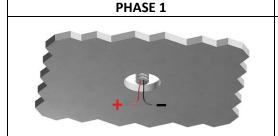
Drill the housing hole for the recess Ø65mm
