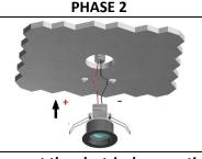
Carry out the electrical connection respecting the cables polarity.
