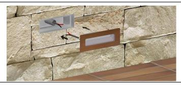
Carry out the electrical connection respecting the cables polarity and with a light pressure insert the Led light body into the formwork
