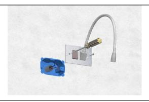
Carry out the electrical connection paying attention to the polarity of the cables and fix the Tulip with two screws
