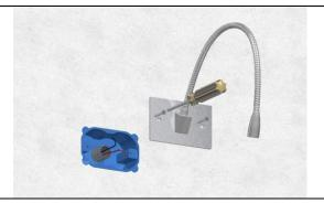
Carry out the electrical connection paying attention to the polarity of the cables and fix the Tulip with two screws
