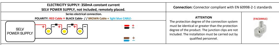
• ATTENTION: Before starting all electrical connections, make sure that the <u>power supply is not powered</u>. The connection to the electricity grid must be carried out <u>only after completing the</u> <u>wiring of all the components</u>. If this simply rule is not respected, the lighting source will be irremediably damaged. The installation must be carried out by qualified personnel.
