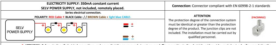
• ATTENTION: Before starting all electrical connections, make sure that the <u>power supply is not powered</u>. The connection to the electricity grid must be carried out <u>only after completing the wiring of all the components</u>. If this simply rule is not respected, the lighting source will be irremediably damaged. The installation must be carried out by qualified personnel.
