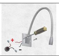
Carry out the electrical connection respecting the cables polarity and fix the lighting body with two screws suitable for the support
