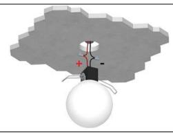
Carry out the electrical connection paying attention to the cables polarity and insert the lamp in seat
