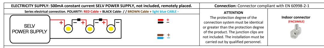
• ATTENTION: Before starting all electrical connections, make sure that the power supply is not powered. The connection to the electricity grid must be carried out only after completing the wiring of all the components. If this simply rule is not respected, the lighting source will be irremediably damaged. The installation must be carried out by qualified personnel.
