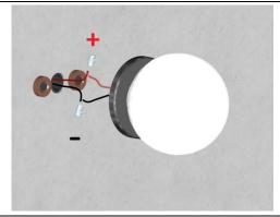
Make the electrical connection paying attention to the cables polarity and put the lamp on the magnets making sure to place them in their seats
