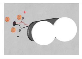
Make the electrical connection paying attention to the cables polarity and put the lamp on the magnets making sure to place them in their seats
