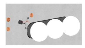
Make the electrical connection paying attention to the cables polarity and put the lamp on the magnets making sure to place them in their seats
