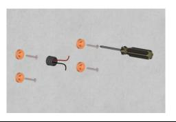
Fix the magnets making sure to respect the measurements of the wheelbases and their perfect coplanarity
