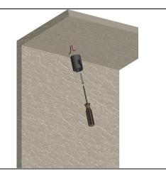
Fix the support to the ceiling with a countersunk screw with maximum diameter 5mm suitable to the support (not supplied by us)
