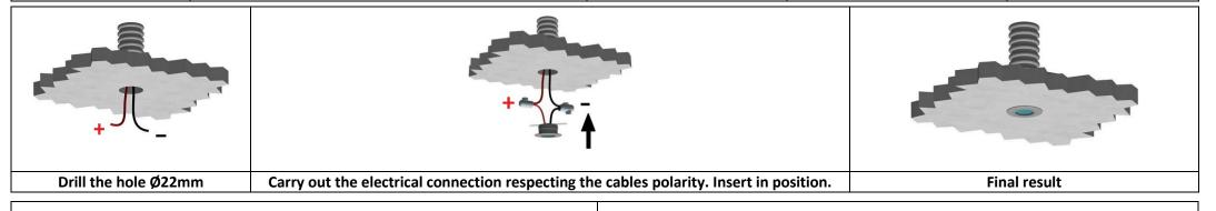
ATTENTION: Before starting all electrical connections, make sure that the power supply is not powered. If this simply rule is not respected, the lighting source will be irremediably damaged.
