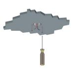
Insert the formwork and fix it to the drywall with two screws
