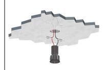
Carry out the electrical connection respecting the polarity. Insert in position the spotlight.
