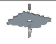
Drill the hole 50mmdiameter for the formwork compartment
