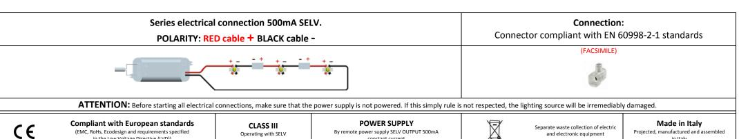
Carry out the electrical connection respecting the polarity. Insert the spotlight in position.
