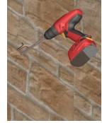
Drill the holes for insertion countersunk screws with maximum diameter 5mm
