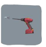
Carry out holes suitable to the wall plugs for countersunk screws with maximum diameter 6mm
